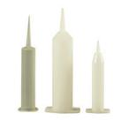
One-piece taper tip molded barrels are made of polypropylene and do not require a dispensing tip to operate. The tapered tip can be cut back to widen the opening and allow more material to flow. The JG30AT (JG30T-1N barrel) has a tip ID of .0385"; the JG30ATL (JG30T-1L barrel) has a tip ID of .170".
