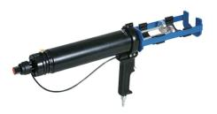
Dual pneumatic gun with a 200 ml capacity for two part applications. The ratio is a dedicated 1:1 (200 ml x 200 ml) and this unit has an adjustable regulator at 100 psi. The maximum output of this gun is 145 psi. Nominal thrust is 484 lbs.
