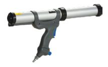
Pneumatic gun has a 10.3 oz. cartridge dispenser that also works for 10 oz. sausage cartridges. It has a series 3 air action system, piston rod action cartridge plunger or sausage, 145 psi max input, and a drawn aluminum barrel.
